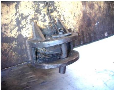
Maintain your recovery points in good condition and ensure they are strong enough. Black Snake engineered round eyes spread the load on pins to avoid high pressure point loading. Weld stronger recovery points on large vehicles by increasing pin/clevis size, use higher grade steel or consult with your equipment supplier for well engineered solutions. Remember that all steel work must be stronger than the recovery strop.
