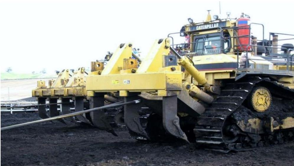
Modified cast fittings supplied by Andromeda Industries Pty Ltd can be installed to one or both ends of the recovery strap. The B fitting is a product well suited for recovery use with bulldozer rippers.
