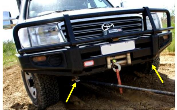
Well engineered light vehicle recovery points match our range of light duty nylon (8t MBS-12t MBS) strops. The photo (left) show an accredited aftermarket tow hitch in place of the towball mount. NEVER USE A TOWBALL! Aftermarket front mounted bullbars must have chassis mounted recovery points. NEVER USE VEHICLE SHIPPING LUGS OR LASHING POINTS!
