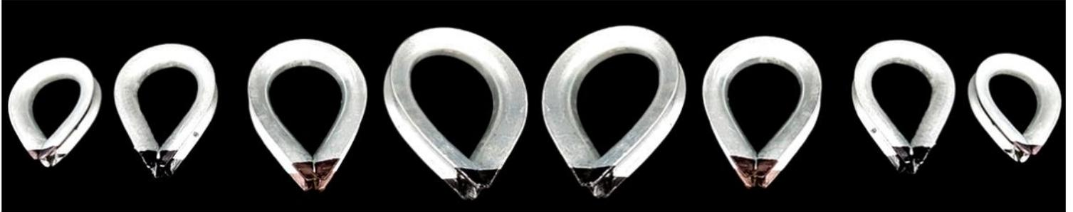
The 10t & 20t MBS Black Snake KEVLAR® range use embedded AS1138 wire rope thimbles. The low elongation properties of the KEVLAR® fibres do not deform wire rope thimbles at these low applied loads. The 30t and 50t MBS Black Snake KEVLAR® range only use AS1138 wire rope thimbles when the knuckles of larger shackles or oversize pins are required.
