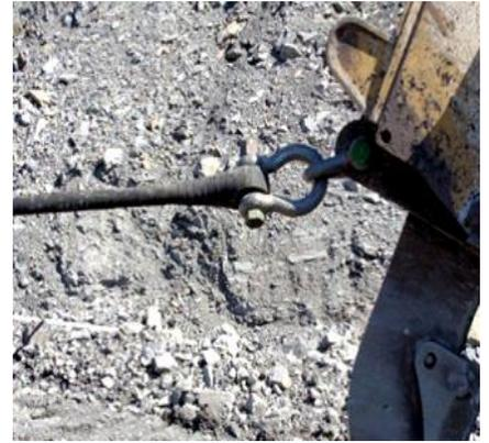
Lugs and pad eyes on the front of mining and road trucks must be linked to the vehicle chassis. Steel plate thickness and hole size should not allow undersize shackles to be mounted or installed. Bolster or cheek plates on lugs can be used to
