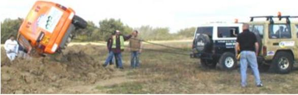
**FLIPPED, NOT BOGGED:** This photo shows recovery of an overturned vehicle which requires very slow uptake of load on the strops and no sudden jerking or high acceleration by the recovery vehicles.
