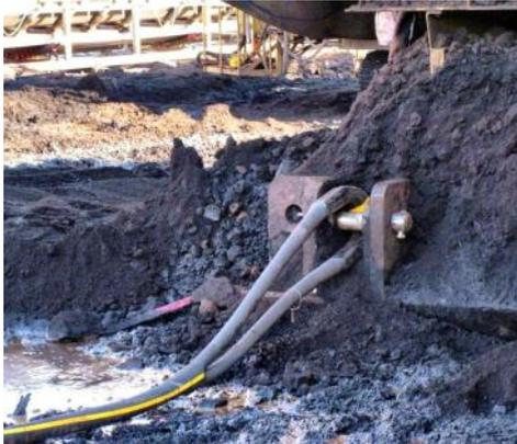
Skid mounted plant and specialized equipment will generally have pin/clevis or inbuilt heavy lugs (pad eyes) with plate thickness and holes designed for shackles of a certain size. Ensure that shackles are correctly matched to the recovery strop. Safety bow shackles (with bolt and nut) are preferable to screw pin shackles. Ensure that personnel are correctly trained to attach these shackles to equipment and strops.
