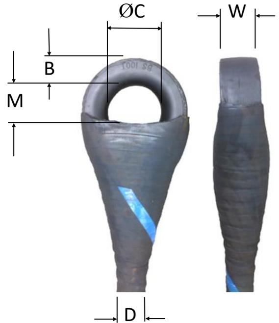
Custom designed and machined eyes are created from high strength, low alloy steel hollow bar. The bore hole is designed to minimize elongation under very high loads and to suit appropriately large shackles. We are always designing for safety and therefore undersized shackles (Jaw width) will not fit on the machined eyes. For example, a 17t S Grade shackle will not fit a 150t stop.
