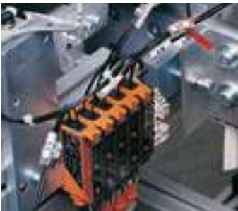
OBF amplifiers can be mounted in areas with limited mounting space
