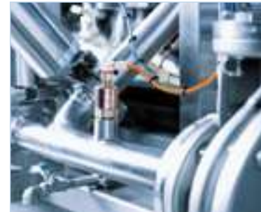
The LMC sensor is ideal for pipe level applications and eliminates obstructions in the flow path that reduce throughput.
