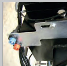
42 Plugs for vehicles factory prepared with VEHH battery cables wiring.
