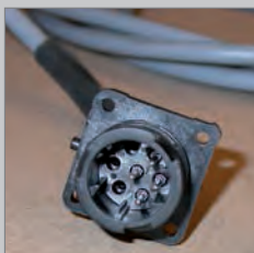
41 Plug for light on cabine showing platform position and on/off switch for vehicles prepared with VEHH wiring.
