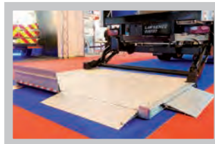
One piece aluminium platform 1800 mm
