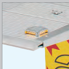
18 Flashing lights on platform.
