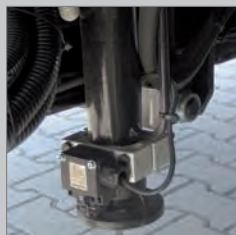
29 Acoustic and illuminated alarm system for hydraulic outriggers.
