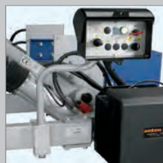
20 Support for the quick assembly of the control box.
