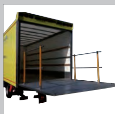
23 Guard hinged and folding on platform.
