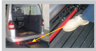
Toe protection bar with micro-switched operation cut-out
