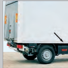
27 Removable hydraulic power pack not integrate with the lift.
