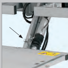
19 Mechanical stop to the body
